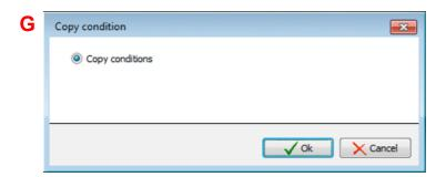
You are dragging a shutdown condition without reference to the "same" WTG. To complete the process, click on OK. If the target object is **empty**, it will be overwritten; if it is **not empty**, the source object will be added as a new object.
