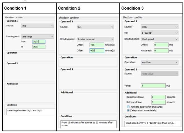
If a shutdown condition is displayed in **red** or **black** bold letters in the display area of the **Special Shutdowns** or **Night shutdowns** window (left half of the window), then SM4 has detected that an input is "not plausible". Please refer to the information in the <u>Plausibilty check</u> section.
