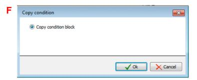
You are dragging a condition block that contains NO shutdown condition with reference to the source WTG (the same WTG). To complete the process, click on OK. If the target object is **empty**, it will be overwritten; if it is **not empty**, the source object will be added as a new object.
