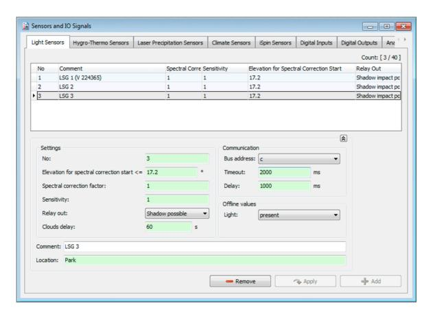
Sensors and IO Signals window, displaying the Light Sensors tab (section)
