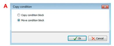
You are moving a condition block within its own WTG block. If you select **Copy condition block**, the condition block will be duplicated (the number of condition blocks increases by 1). If you select **Move condition block**, nothing will change except for the position of the block.
