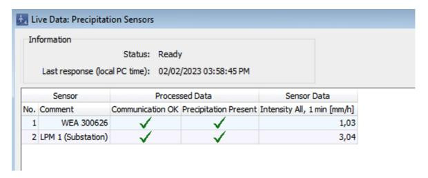
Live Data: Laser Precipitation Sensors window (section)
