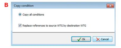
You are copying a WTG block that contains one or more shutdown conditions with reference to the source WTG (the same WTG). If a checkmark is set, the reference will be replaced with a reference to the target WTG (this is typically used), otherwise the reference to the source WTG will remain unchanged.
