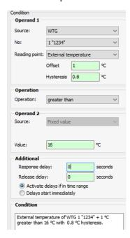
Click on **Add** at the bottom right in the window and then define the second condition for **Condition block 1** in the **Conditions** input area as follows:
