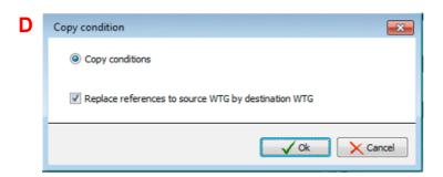
You are copying a shutdown condition with reference to the source WTG (the same WTG). If a checkmark is set, the reference will be replaced with a reference to the target WTG (this is typically used), otherwise the reference to the source WTG will remain unchanged.
