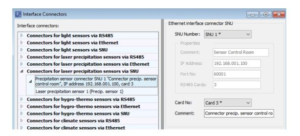
3. Add the appropriate sensors to the previously created interface connector, see also <u>Interface</u> <u>connector window</u> and the following screenshot:
