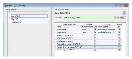
Under **Settings**, **Column Header** now enter the desired abbreviations for the reading points and activate the boxes under **Unit**, see the following screenshot:
