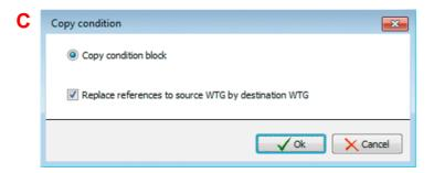
You are copying a condition block that contains one or more shutdown conditions with reference to the source WTG (the same WTG). If a checkmark is set, the reference will be replaced with a reference to the target WTG (this is typically used), otherwise the reference to the source WTG will remain unchanged.
