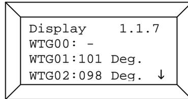
The nacelle position transmitted e.g. from the wind park server may be adjusted for each WTG according to a user-settable offset value.
