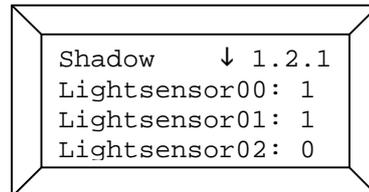
The function of the light sensors is to determine the direct portion of the visible sunlight. Actual shadow impact is possible only if the direct portion is high enough. Menu 1.2.1 provides information on the light conditions at the respective light sensor. A status of 1 means that due to the light conditions, actual shadow impact is possible. With a status of 0, this is not possible.
